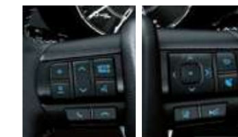
Steering wheel switches: The 4-direction switch integrated in the steering wheel makes it easy to adjust the multi-information display among other functions
